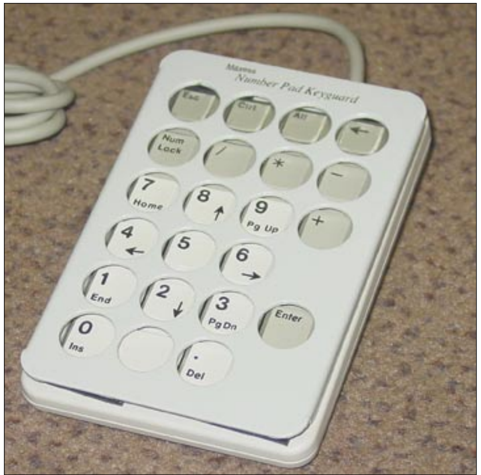
Cherry Numeric Keypad and Keyguard (Inclusive) can be attached to any Windows keyboard for placement on the left or any where the user is more comfortable.
